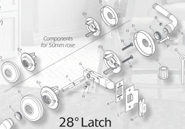
N - Thru-Bolt Machine Screws With Locking Washer (2)
