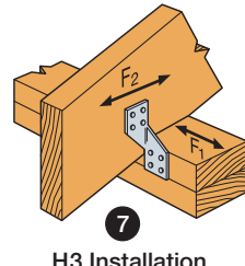
H3 Installation (nails into upper top plate)
