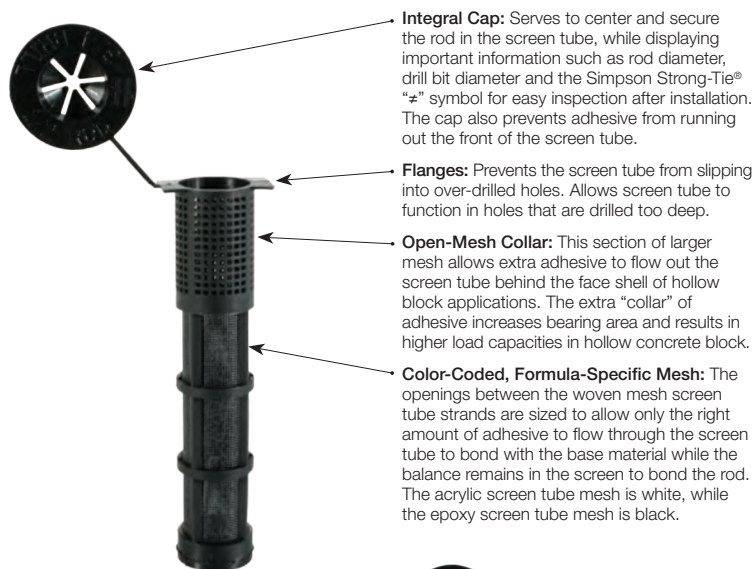
Epoxy Adhesive Screen Tube (mesh is black)
