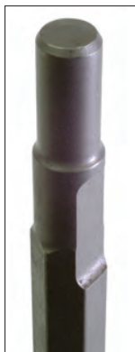
Spline (design disables rotohammer rotation)
