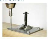
The innovative Take-Up Washer (TUW) plays a key role in the long-term performance of the SDWF when installed between the screw head and the sole plate of the upper floor. As the structure settles because of shrinkage and construction loading, the threaded portion under the head of the screw ratchets up through the tabs of the TUW, which is fastened with Simpson Strong-Tie Strong-Drive SD screws.
