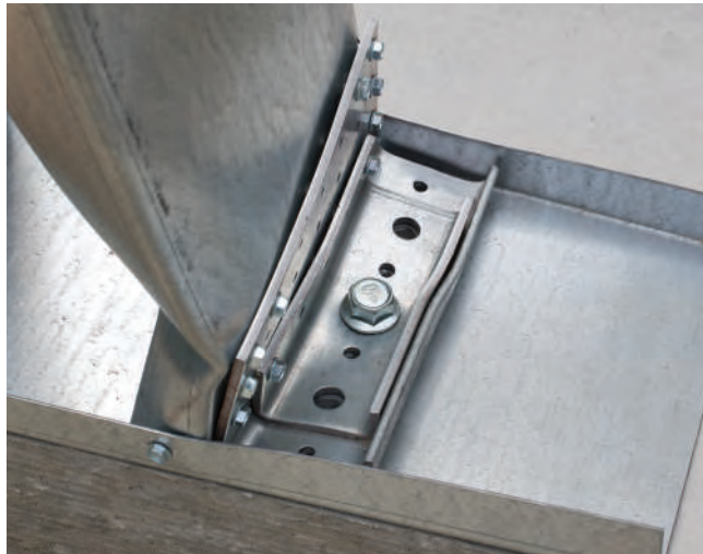
RCKW assembly test with member failure.
