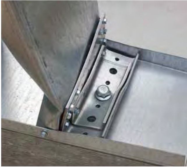
RCKW assembly test with member failure.
