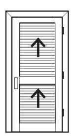
When the Blind Side is on the Stop Side, the Louvers run up, meaning you can see into the next room.
