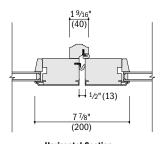
**Horizontal Section** Astragal, Lead Panel-Lead Panel
