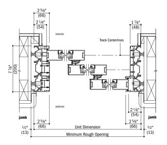
**Horizontal Section** Three-Panel, One-Direction Panel Operation
