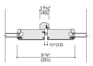
**Horizontal Section** Astragal, Lead Panel-Lead Panel
