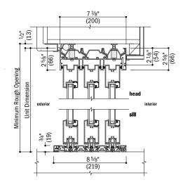
**Vertical Section** On-Floor Drainage Sill
