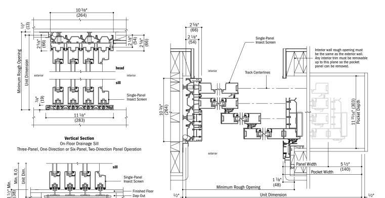
Vertical Section Flush Sill Horizontal Section
