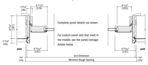
**Horizontal Section** Hinge Jamb, Hinge Jamb
