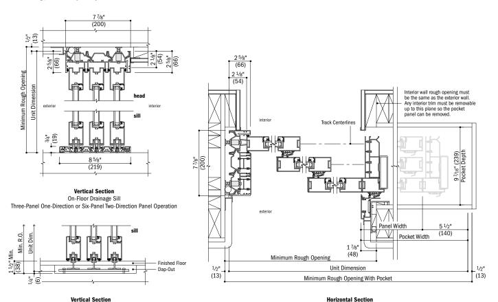
Flush Sill Three-Panel, One-Direction or Six-Panel, Two-Direction Panel Operation
