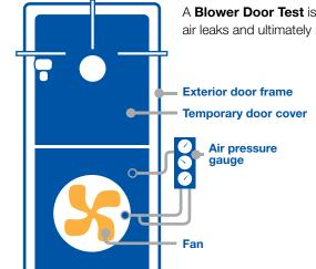
A **Blower Door Test** is conducted to pinpoint where buildings are losing energy, It's all about locating air leaks and ultimately making new and old buildings more energy-efficient.
