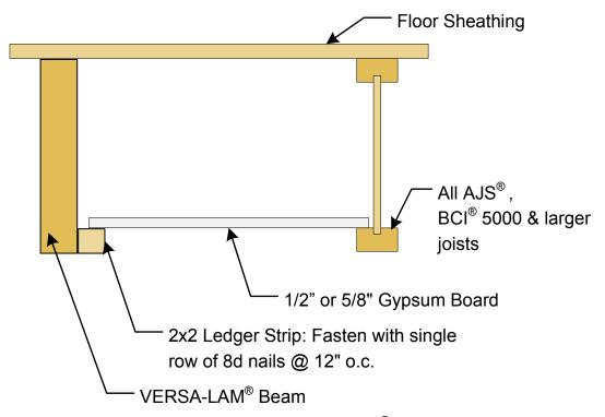
Note: Detail may be used between two VERSA-LAM® beams as well, though floor protection not required between two VERSA-LAM® beams/joists (1 ½" x 9 ¼" or greater sizes) per 2012 IRC R501.3 and 2015 IRC R302.13, exception 4.
