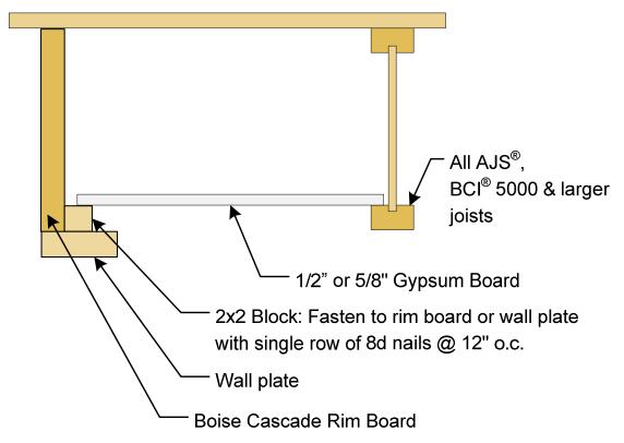
Note: In conditions where perpendicular blocking is installed between endwall and first floor joist, install gypsum board between blocking panels.
