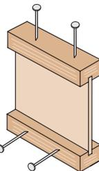
Nailing Parallel to Glue Lines (Narrow Face)
