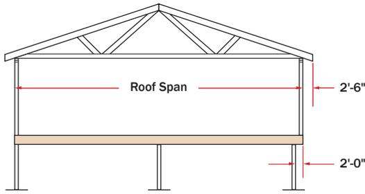
The detail to the right on this page shows the installation of cantilever reinforcement for load-bearing cantilevers up to a maximum length of 2'-0". Cantilevers longer than 2'-0" cannot be reinforced. **However, longer cantilevers with lower loads may be allowable without reinforcement. Analyze specific applications with the BC CALC® software.**
