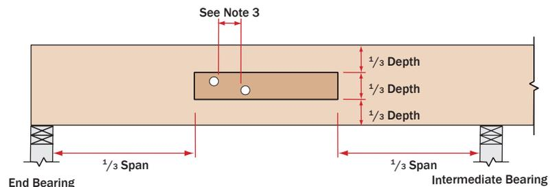
6. These limitations apply to holes drilled for plumbing or wiring access only. The size and location of holes drilled for fasteners are governed by the provisions of the *National Design Specification® for Wood Construction*.
