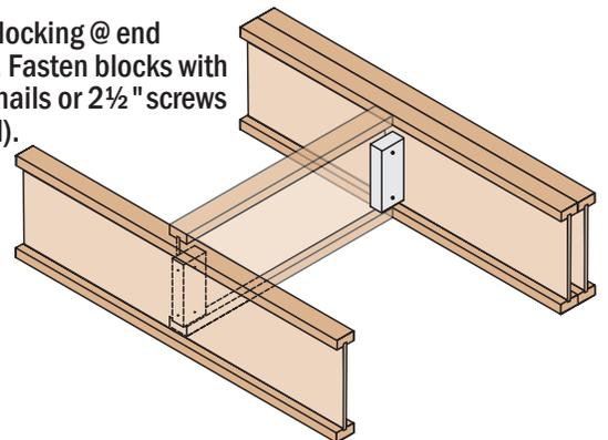
Attach floor panel to each blocking panel with (3) 8d nails, minimum.
