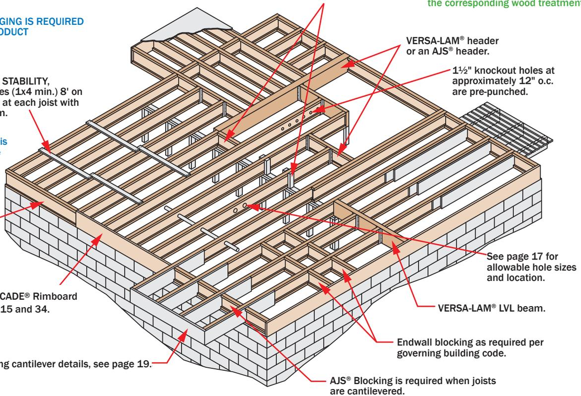
BCI® Joists, VERSA-LAM® and ALLJOIST® must be stored, installed and used in accordance with the Boise Cascade EWP Installation Guide, building codes, and to the extent not inconsistent with the Boise Cascade EWP Installation Guide, usual and customary building practices and standards. VERSA-LAM®, ALLJOIST®, and BCI® Joists must be wrapped, covered, and stored off of the ground on stickers at all times prior to installation. VERSA-LAM®, ALLJOIST® and BCI® Joists are intended only for applications
