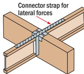
See connector manufacturer's code evaluation reports and literature for allowable loading. Axial force in top flange shall be considered in AJS® joist design.
