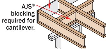
For load bearing cantilever, see page 19. Uplift on backspan shall be considered in all cantilever designs.
