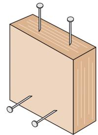
Nailing Perpendicular to Glue Lines (Wide Face)
