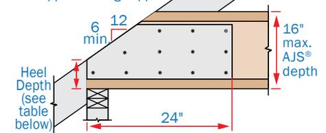
2x blocking required at bearing (not shown for clarity). <sup>23</sup>/<sub>32</sub> min. plywood/OSB rated sheathing as reinforcement. Install reinforcement with face grain horizontal. Install on both sides of the joist, tight to bottom flange. 1/4" gap between reinforcement and bottom of top flange. Apply construction adhesive to contact surfaces and fasten with 3 rows of min. 10d box nails at 6" o.c. Alternate nailing from each side and clinch.
