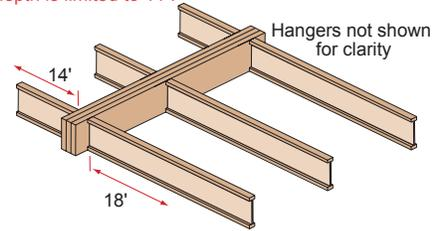
Find: A multiple 1 1/4" ply VERSA-LAM® that is adequate to support the design loads and the member's proper connection schedule.
