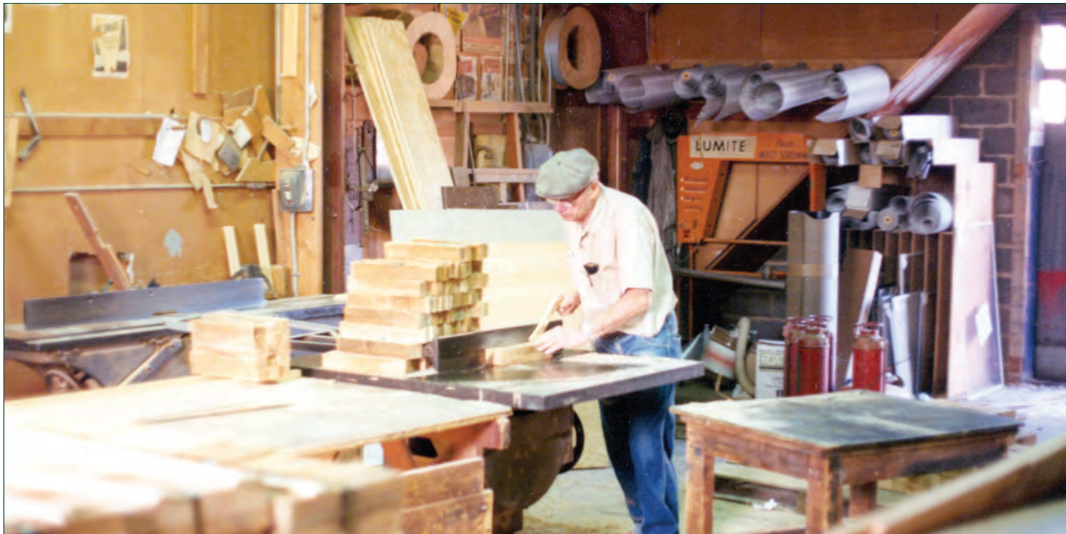
Circa 1977 - Chris Schroeder in the Fair Lawn Millwork Shop. Chris is milling oak hubs, which would be used by surveyors for stakes. "We used to make them by the thousands" recalls Doug Kuiken. Sold for approximately $10 a bundle.
