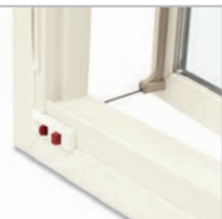
CASEMENT WOC D Limits opening to 4" while providing for full egress. ASTM F2090-10 compliant.
