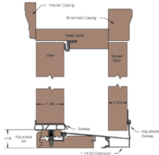
Non-Impact Prehang Details with Standard Jamb and Inswing Sill and Storm Door Attached
